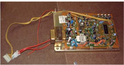
My original NTSC card. I installed the molex connector. I'm not sure where the other red wire is supposed to go.
