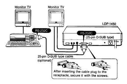
Interface cable to be connected to the RS-232C 25-pin D-SUB type connector must be shielded as follows.
